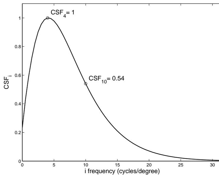
Fig. 1. Contrast Sensitivity Function (CSF) of Nygan et al. [28]. The slopes of two particular sensors respectively tuned to low-frequency stimuli ( $CSF_4 = 1$ ) and high-frequency stimuli ( $CSF_{10} = 0.54$ ) have been highlighted.
