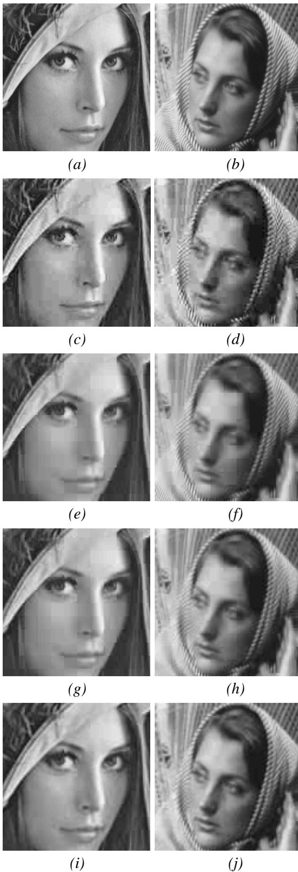
Fig. 5. Examples of decoded images. (a) Lena, and (b) Barbara (zoom of the original images at 8 bits/pixel). The bit-rate for these examples is 0.3 bpp (27:1) (Lena) and 0.4 bpp (20:1) (Barbara). (c) and (d) JPEG, (e) and (f)  $\varepsilon$ -SVR, (g) and (h) RKi-1, and (i) and (j) CSF-SVR.
